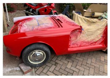
After a disastrous first attempt at applying the colour, when I had the spray gun set up completely wrong and had to sand off the paint I'd applied. I have now got my act together and sorted the gun. The photos of the nearside wing and door show a nice shiny finish. I'll now move the car over to the other side of my narrow garage, apply a bit of high-build primer and several coats of red gloss.
